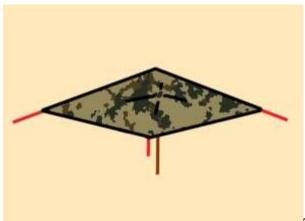
This type of shelter is very similar to the basic sunshade shelter but it adds a central support pole at the tarp's midpoint. It is designed for rain or snow runoff and it's pretty sturdy if you secure the four corners of the tarp well enough. You can make it as tall or as short as you need depending on the length of the pole. This shelter provides a great runoff for rain or snow, but it doesn't have any sides to protect you from the wind or cold.
